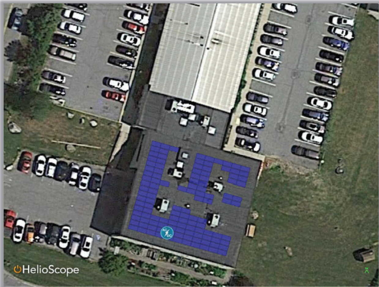
Figure E18.7: Site diagram/illustration that includes location/design of array, and proposed capacity (47.6 kWdc)
