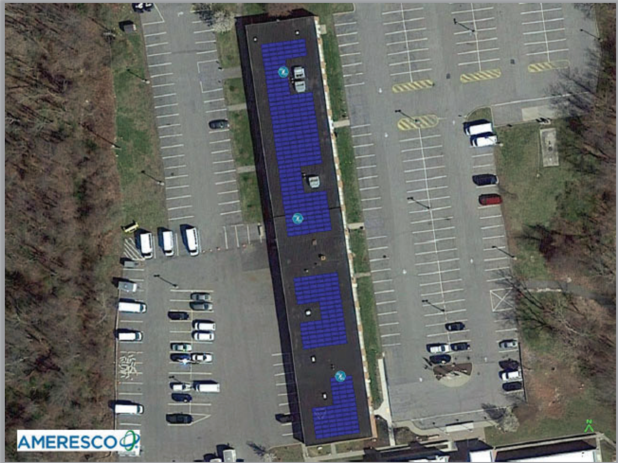
Figure E18.6: Site diagram/illustration that includes location/design of array, and proposed capacity (131.4 kWdc)
