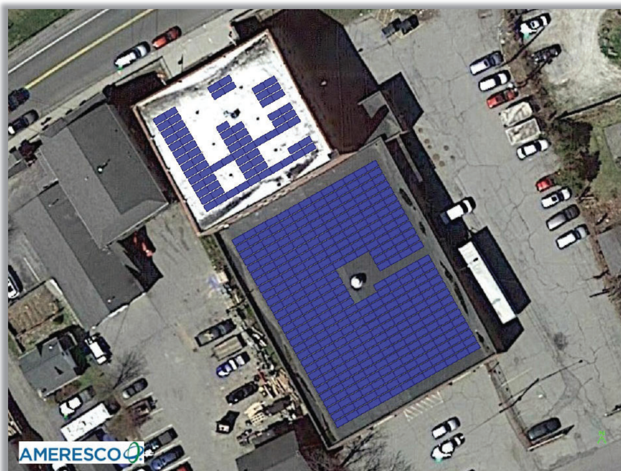
Figure CNR18.1 Site diagram/illustration that includes location/design of array, and proposed capacity (152.9 kWdc)
