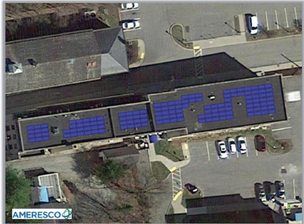
Figure E18.2: Site diagram/illustration that includes location/design of array, and proposed capacity (45.6 kWdc)
